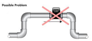
Allows air pockets to form at sensor
